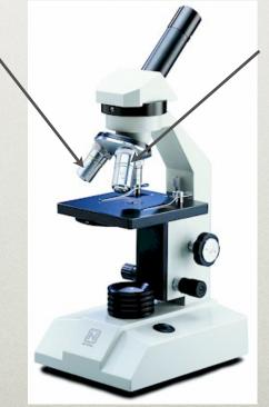
• These 2 clips hold the slide in place on the stage.
